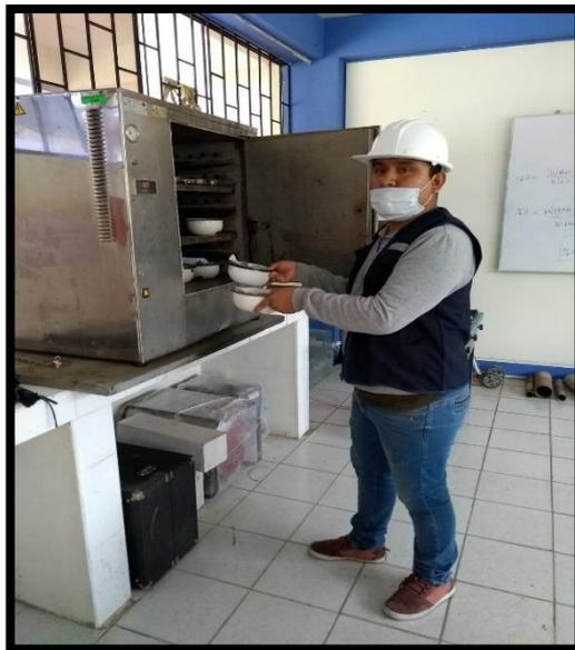
**FIGURA 22: LA PIEDRA SE DEJA SECAR EN EL HORNO****GRAVEDAD ESPECIFICA Y ABSORCION:**
