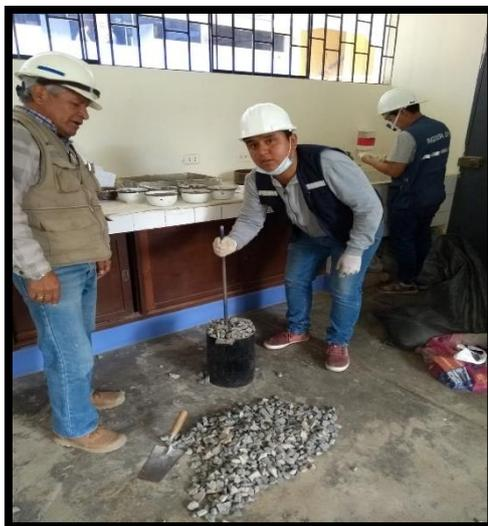
**FIGURA 21: LA PIEDRA SE DEJA CAER A CIERTA ALTURA COMPACTANDO Y CHUCEANDO EN TRES CAPAS IGUALES, ENRASANDO Y PESANDO LA MUESTRA**
