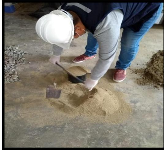
**FIGURA 14: LA ARENA SE DEJA CAER A CIERTA ALTURA SIN COMPACTAR, ENRASANDO Y PESANDO LA MUESTRA**
