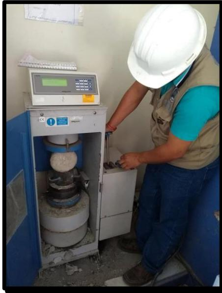
**FIGURA 39: ROTURA DE LA PROBETA, PARA COMPROBAR
