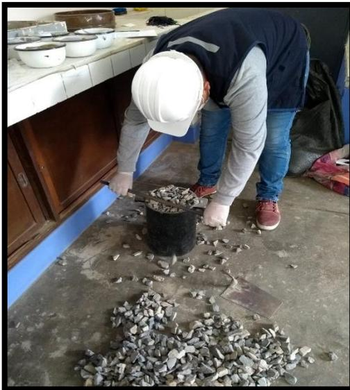
**FIGURA 20: LA PIEDRA SE DEJA CAER A CIERTA ALTURA SIN COMPACTAR, ENRASANDO Y PESANDO LA MUESTRA**
